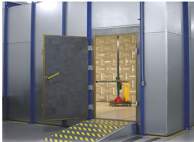
FIGURE 3. A chamber without a pit requires an equipment ramp. A swinging door lined only with ferrite tiles will clear the door opening. Courtesy of Panashield.
